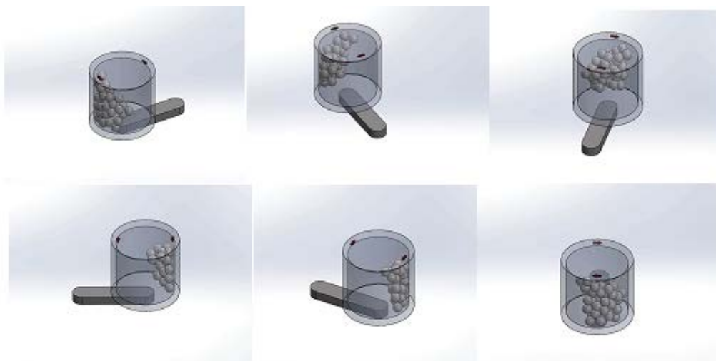
Fig. 2 – Fragments of motion of 32 balls grouped into tetrahedrons
