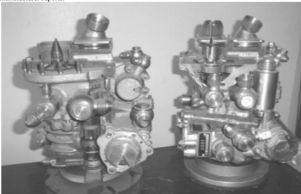
Fig. 1. Gear pumps fuel-supply system of aircraft engines AI-25 and AI-25T: 1 - unit, 2 - unit, 3 - pair friction "ends of gear teeth - saddle."
