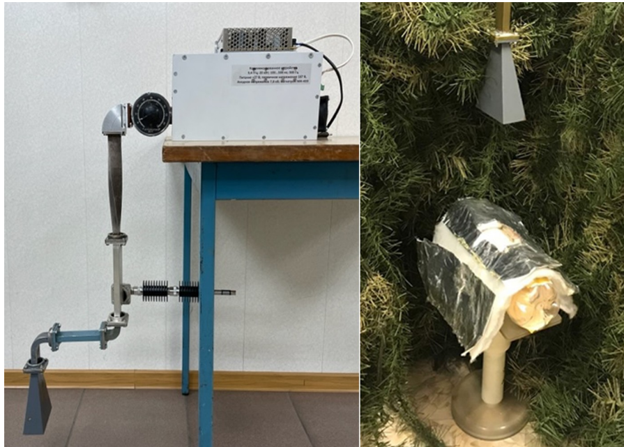
Figure 5 - Stand for location and irradiation of a biological object DOI: https://doi.org/10.23670/IRJ.2024.139.11.5
