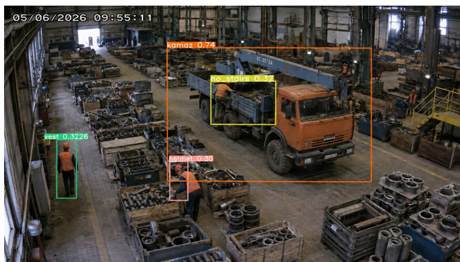
Figure 1 - Detection of a violation: climbing into a KamAZ truck bed without a ladder
