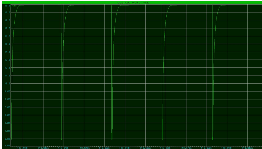
Figure 5 - Graph representing the voltages at the output of the multivibrator DOI: https://doi.org/10.60797/IRJ.2026.166.38.6
