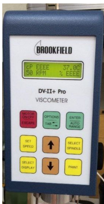
Figure 1 - The Brookfield DV-II+PRO viscometer DOI: https://doi.org/10.60797/IRJ.2025.161.18.1
