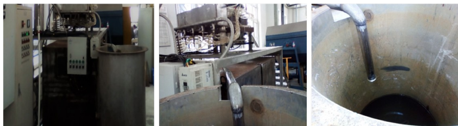
Figure 8 - Water-bubbling gas purification system, formed during the melting of ash waste from incineration DOI: https://doi.org/10.60797/IRJ.2025.154.58.10
