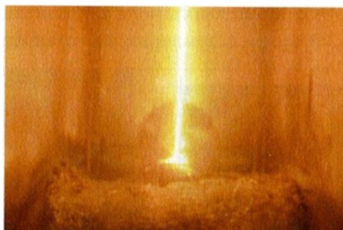
Figure 6 - Discharge of the melt jet from the reactor vessel and its casting into molds
