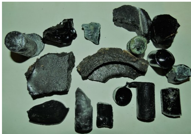
Figure 7 - Examples of cast materials (tiles and cylinders in section) obtained from the melt DOI: https://doi.org/10.60797/IRJ.2025.154.58.9
