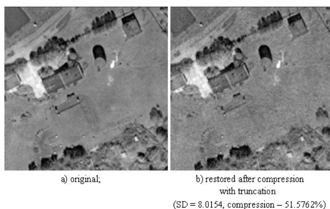
Figure 4 - Images using compression of the spatio-spectral representation based on the SSR DOI: https://doi.org/10.60797/IRJ.2024.146.35.4
