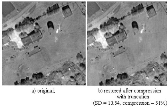
Figure 3 - Images using compression of the spatial spectral representation based on Walsh functions
