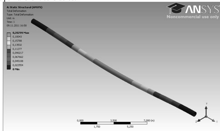
Fig. 5. The deformations in a gas pipeline in soil settlement conditions
