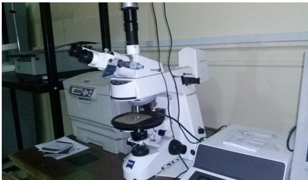
Fig. 1 – Zeiss Axioskop 40 Micro Hardness Tester MHT 10
